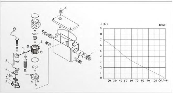
The 250 is a small gray water pump that may be used to pump waste water away from a shower, sink, bar sink, or other fixture.
