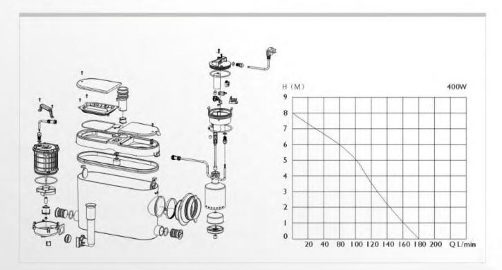
Designed to provide easy access for greywater pumping applications such as kitchens and utility rooms, convenient covers allow simple service and maintenance of the pump without having to remove it.
