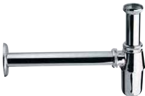
970 Z Sifone a bottiglia in zama senza pilettina, per lavabo, 1" 1/4, 1" 1/2, canotto cm. 30. Bottle trap in zamac without waste, for wash-basin, 1" 1/4, 1" 1/2, outlet tube cm 30.
